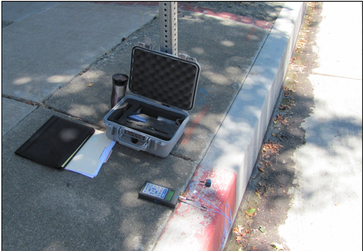
Figure 2 – Vibration Monitoring Equipment Setup
