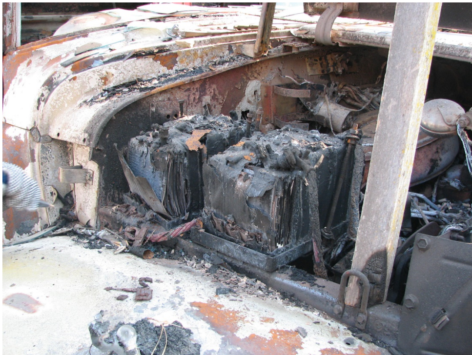
Battery inside burnt vehicle.
